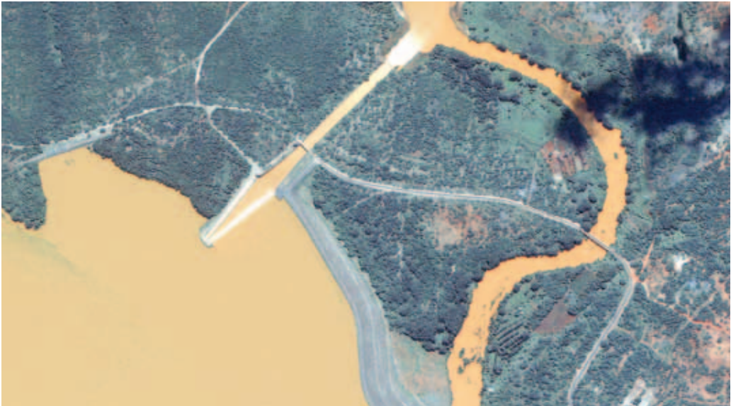
Google Earth image of the outflow of the Masinga Dam and the Masinga Power Station, on the Tana River, in November 2003, during the short rainy season Note: The Masinga Dam has been well documented as suffering from severe siltation resulting from deforestation activities upstream
