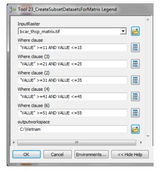
Upon running the Tool, each 'where clause' produces a raster each with 5 classes. The first raster that is created using the 'where clause' "VALUE" >=11 AND "VALUE" produces a raster containing values 11,12,13,14 and 15. This shades the first column of the matrix legend as illustrated below from 11-15, representing:
