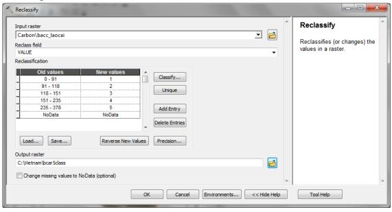
The Result of reclassification of biomass carbon is presented here: Each of the classes has been assigned a new value from 1-5.
