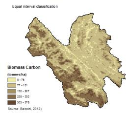
**a.** Add the dataset to be used for the **x-axis** into ArcMap i.e. in this example the **biomass carbon dataset.** Decide on a classification scheme and symbolise the data into 5 classes. The **quantile** is often the best method to show the variation in pattern of carbon distribution (see maps above).
